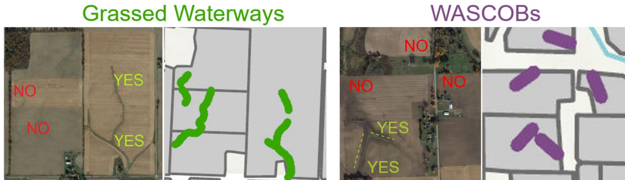
Figure 3. Example fields analyzed in priority subwatersheds depicting absence (“NO”) and presence (“YES”) of grassed waterways (left, green) or WASCOBs (right, purple) in approximate locations suggested by ACPF.
