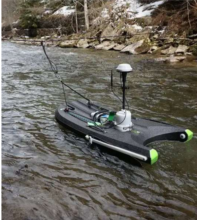
Figure 5-8. Sontek RiverSurveyor M9 ADCP.
